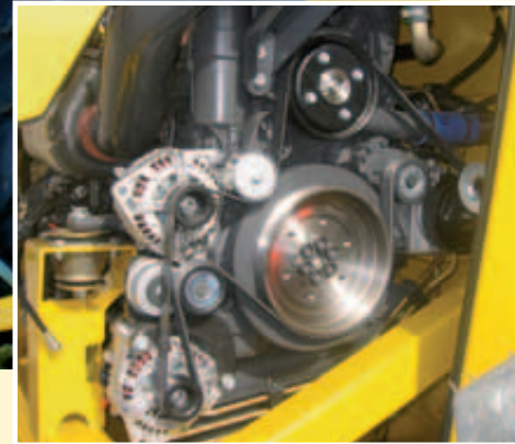
Low maintenance auto tension belt drive
