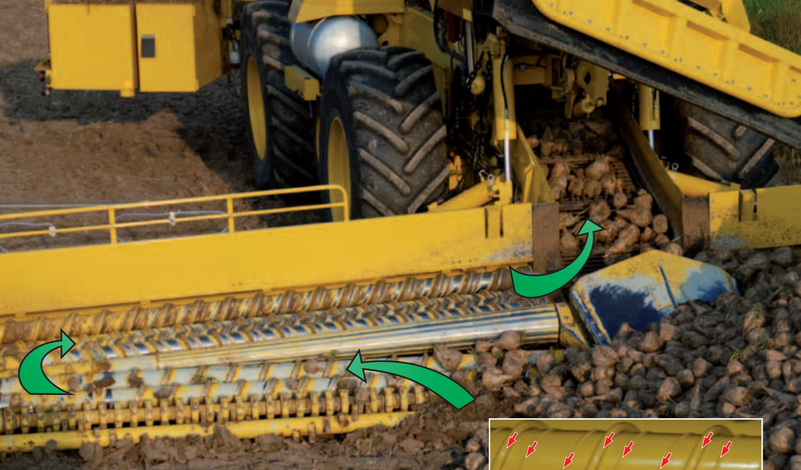
Double cleaning path – conical roller separates the beet flow
