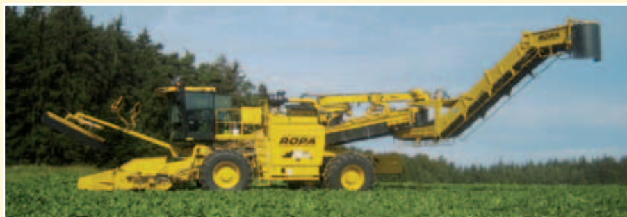
Standard loader, 11.5 m loading reach
