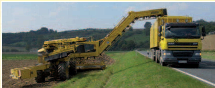
Extended loader, 13 m loading reach
