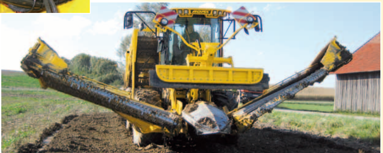
Change-over to transport mode in only 2 minutes without the operator having to leave the cab
