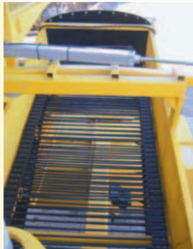
Transfer conveyer cleaner
