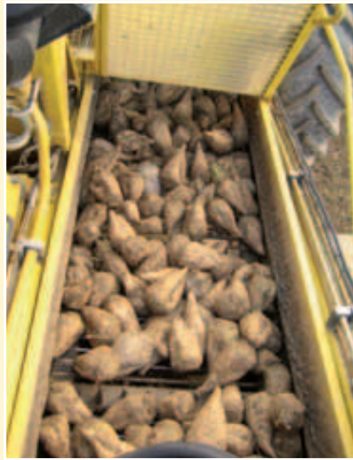
In-feed web with durable PU-collection cleats
