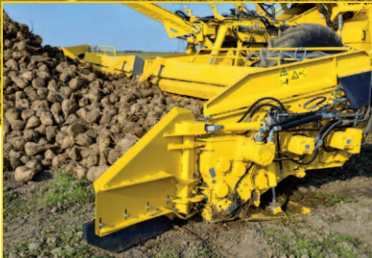
Separate drives for 3 groups of rollers with individual setting of revolutions and automatic reversing for stone protection
