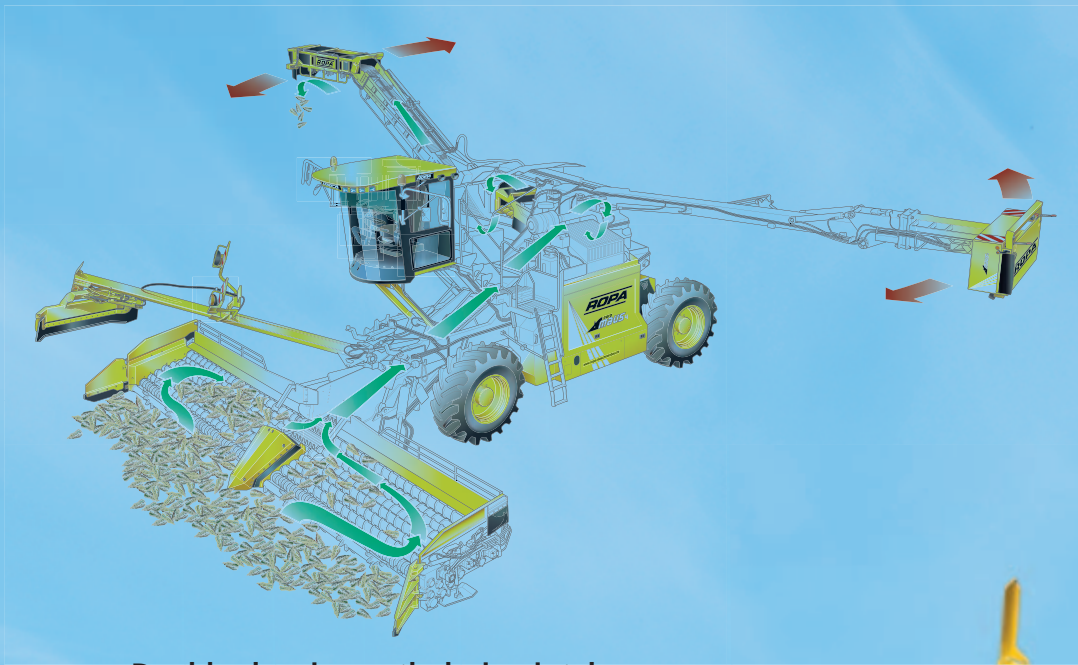
Double cleaning path during intake - individually adaptable cleaning intensity
