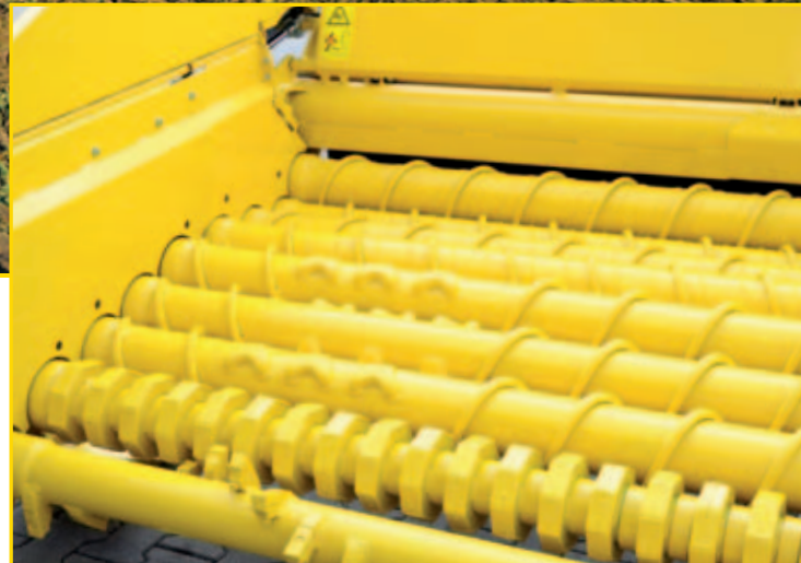
Separate drives for 3 groups of rollers with individual setting of revolutions and automatic reversing for stone protection
