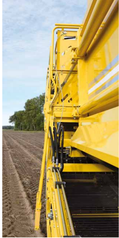
Working platform, 300 mm extendable - immense working area allows freedom of movement
