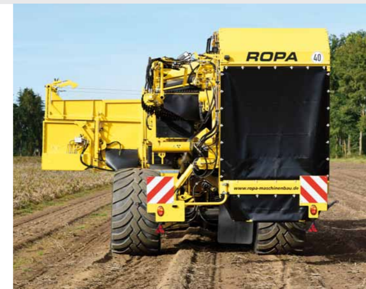
Standard hydraulic slope compensation - optimised cleaning and greater comfort for pickers
