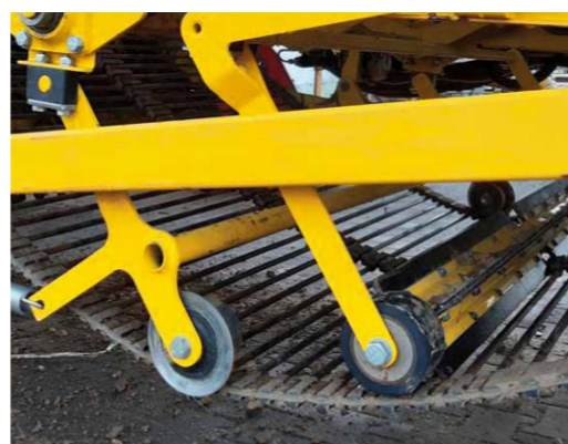
Sieve conveyor tensioner with a separate, retractable cleaning roller
