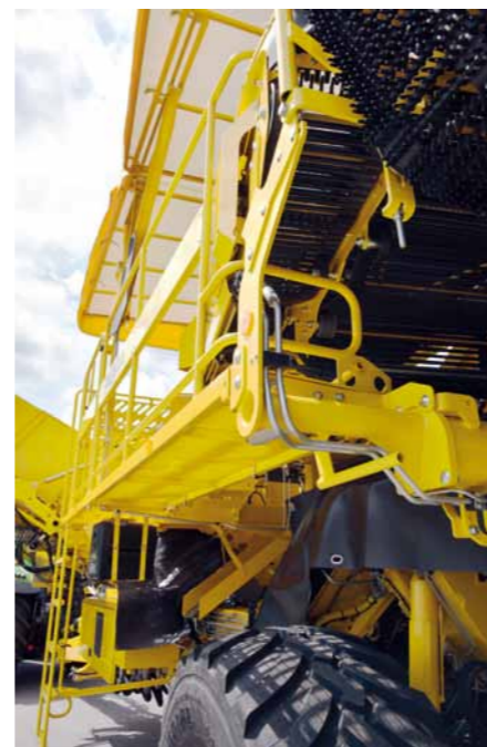
Sorting platform can be swung out for even more space
