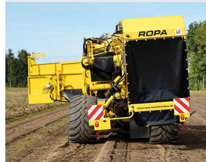
Standard hydraulic slope compensation - optimised cleaning and greater comfort for pickers
