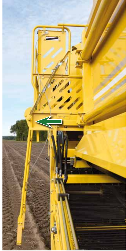
Working platform, 300 mm extendable - immense working area allows freedom of movement
