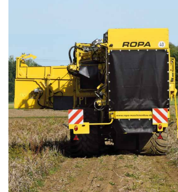
Lifting on tracks with retracted telescopic axle - does not run over the potato ridge
