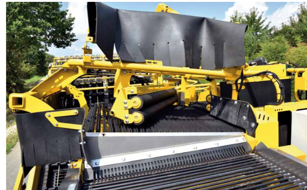
Keiler 2 4 pintle belts with deflector rollers
