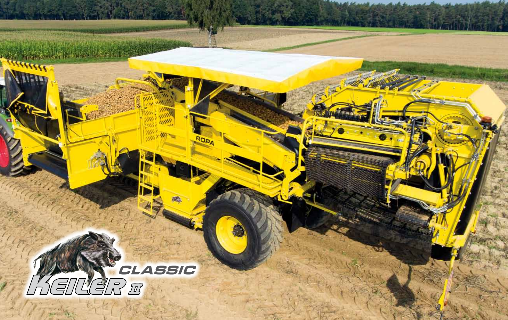
Sorting platform can be swung out for even more space
