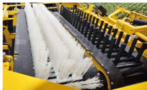
Combined finger comb and brush comb
