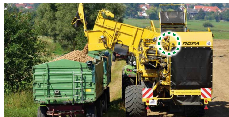
Additional cameras for sieve conveyor, leaf chain, pintle belt, picking table, bunker and reversing
