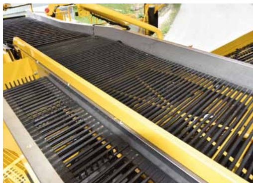
Removable picking table elevation
