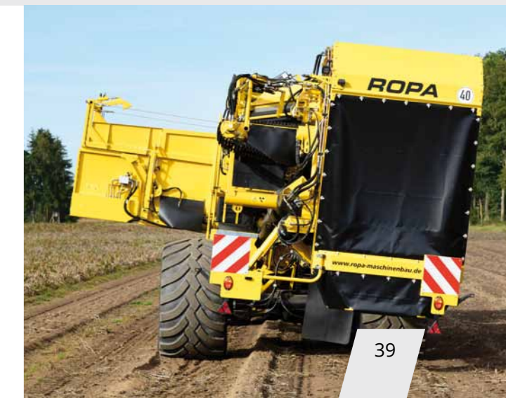
Standard hydraulic slope compensation - optimised cleaning and greater comfort for pickers
