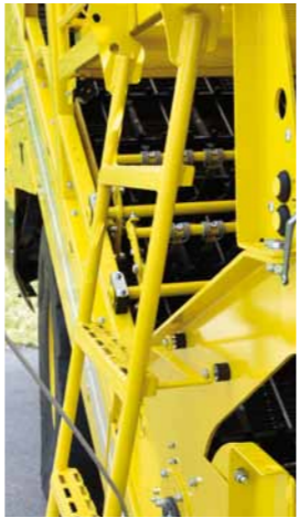
Folding ladder damping for safe access
