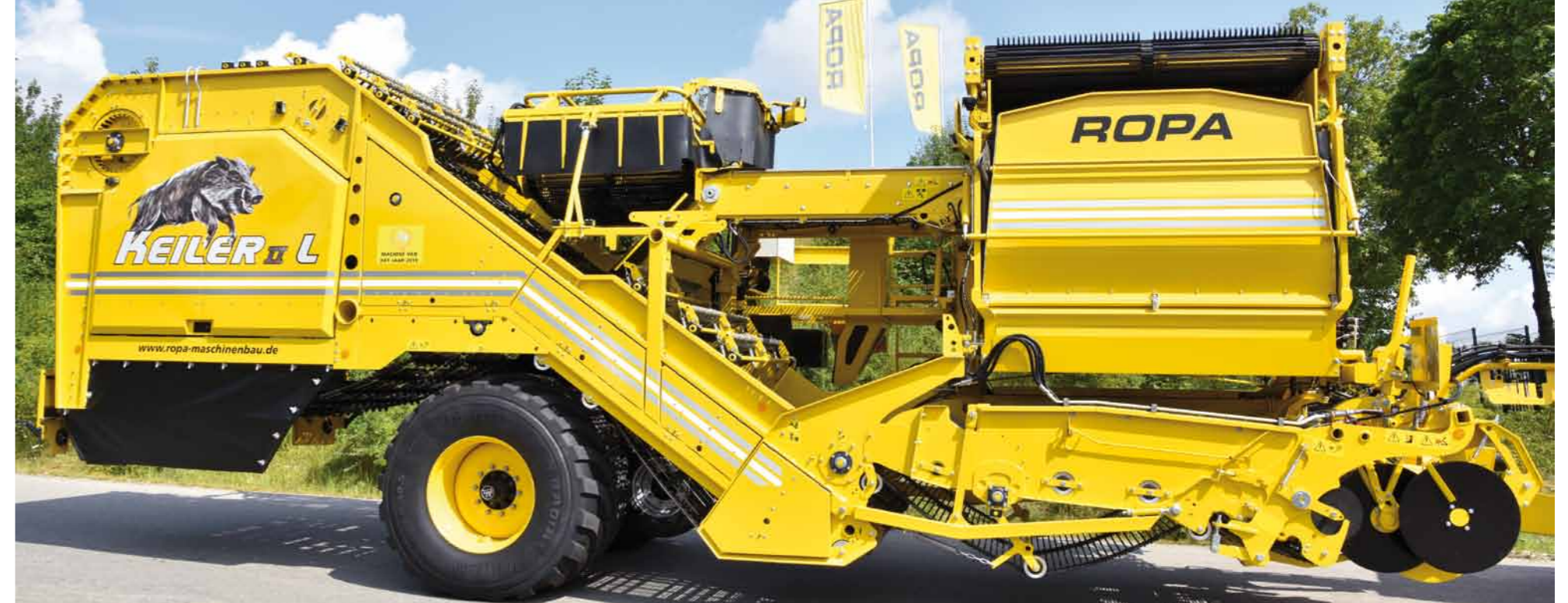
Keiler 2 L 4 pintle belts without trash conveyor and without sorting platform on the right
