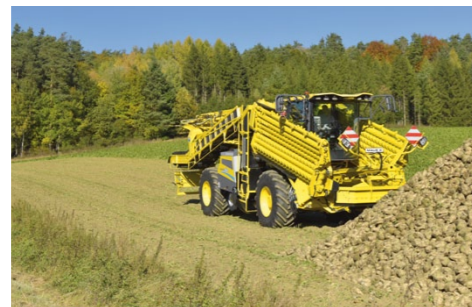
Separate drives for 3 groups of rollers with individual rotational speed adjustment and automatic reversing for stone protection. All rollers are hard-welded as standard.
