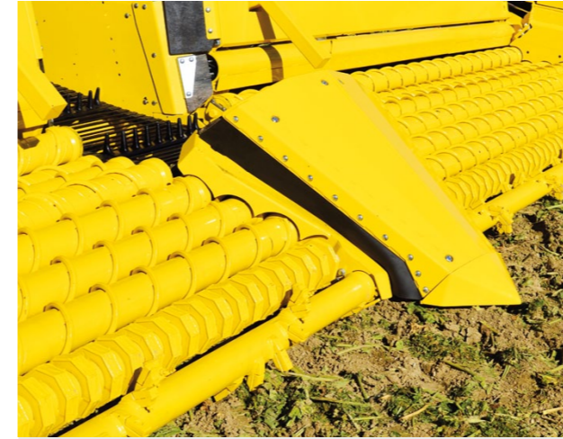
The central mark with its replaceable cone and a split cap has a free-of-play drive designed with conical bearing and automatic lubrication.
