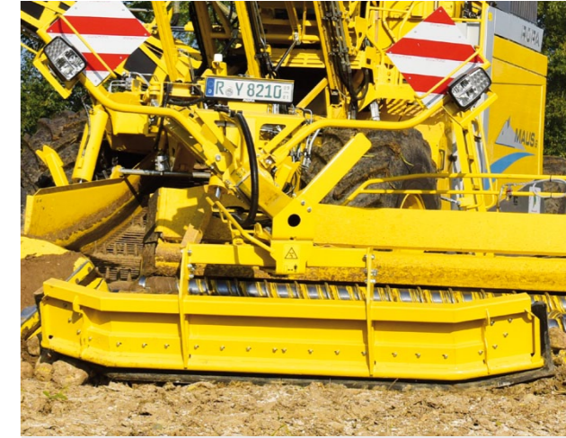
Pile pickup and residual beet pickup with angled corners and reinforced rubber lip.
