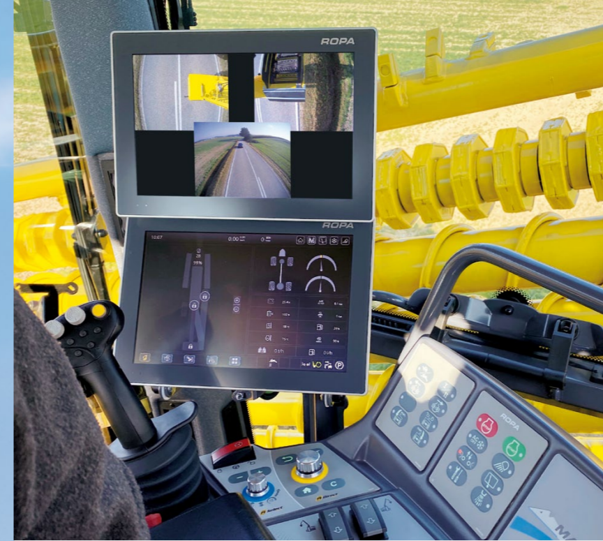
R-View with rear view camera and two side cameras. Each camera can be zoomed in to full screen at the touch of a finger.
