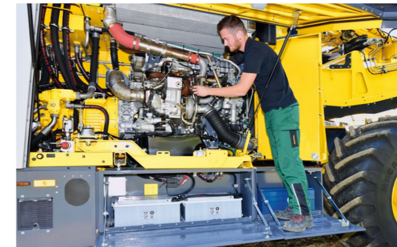
The Mercedes-Benz OM936 engine is driven at strongly reduced engine rpm during loading (possible from 1,150 rpm), while enough power is preserved for extreme conditions.
