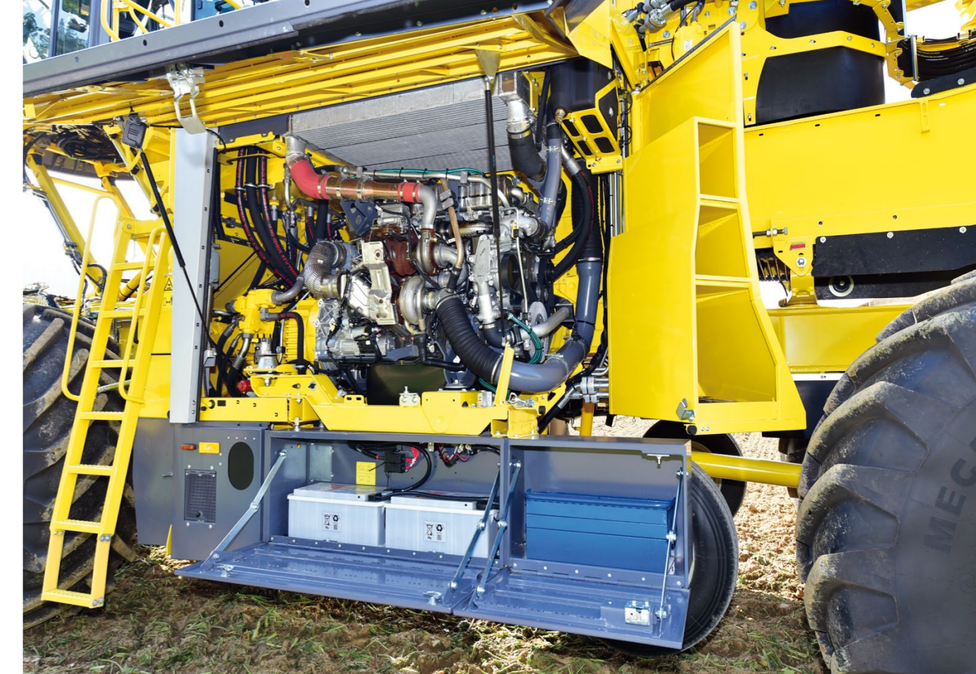
The Mercedes-Benz OM936 engine is driven at strongly reduced engine rpm during loading (possible from 1,150 rpm), while enough power is preserved for extreme conditions.
