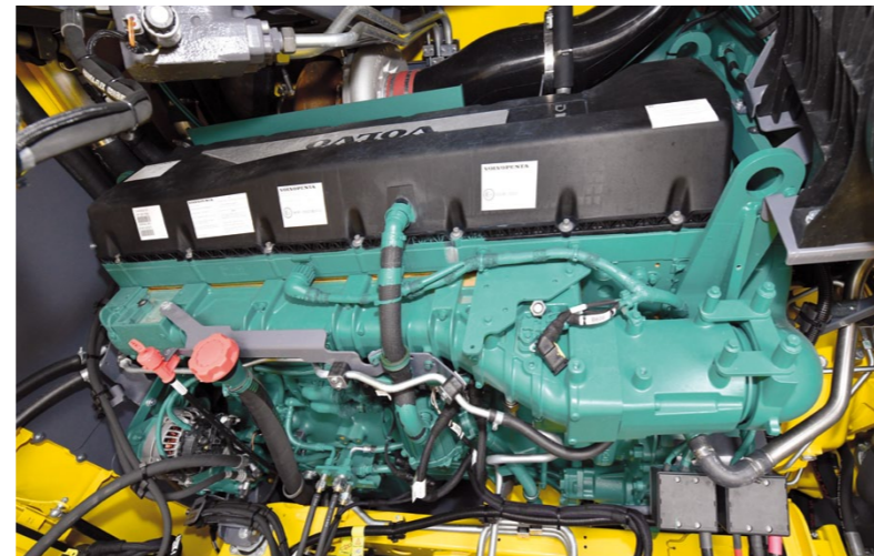
Volvo Penta TWD1683VE is the basis for greater daily output at less fuel consumption and even more power at lower speeds.
