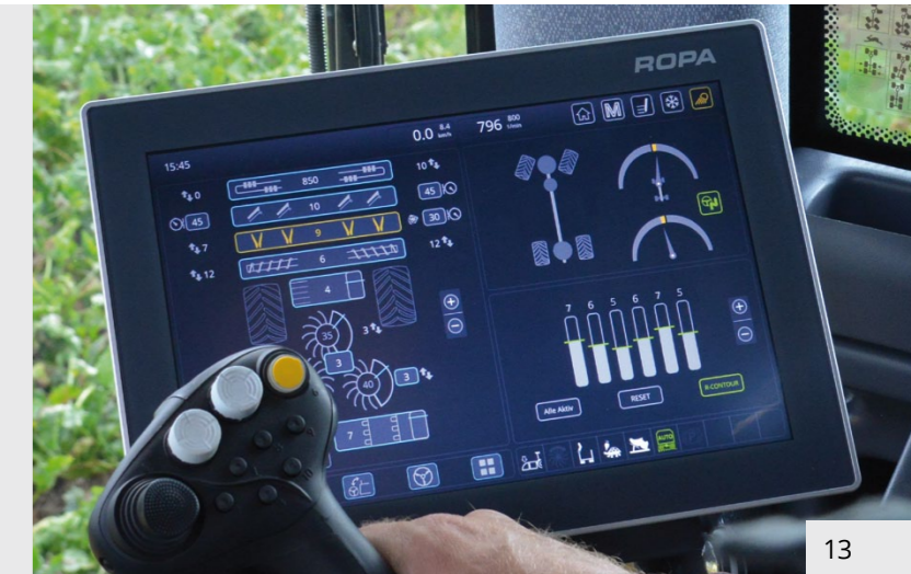
Automatic share depth adjustment for uneven ground contour Ultrasonic sensors beside every beet row record the ground surface contour
