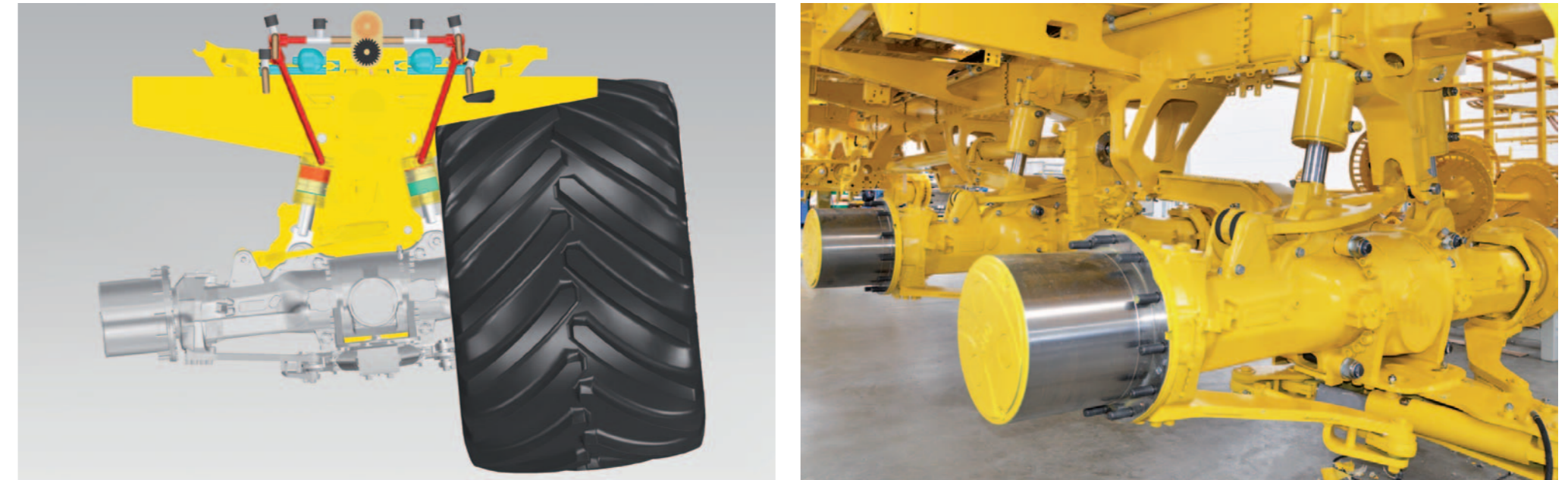
Hydraulic chassis, automatic slope compensation
