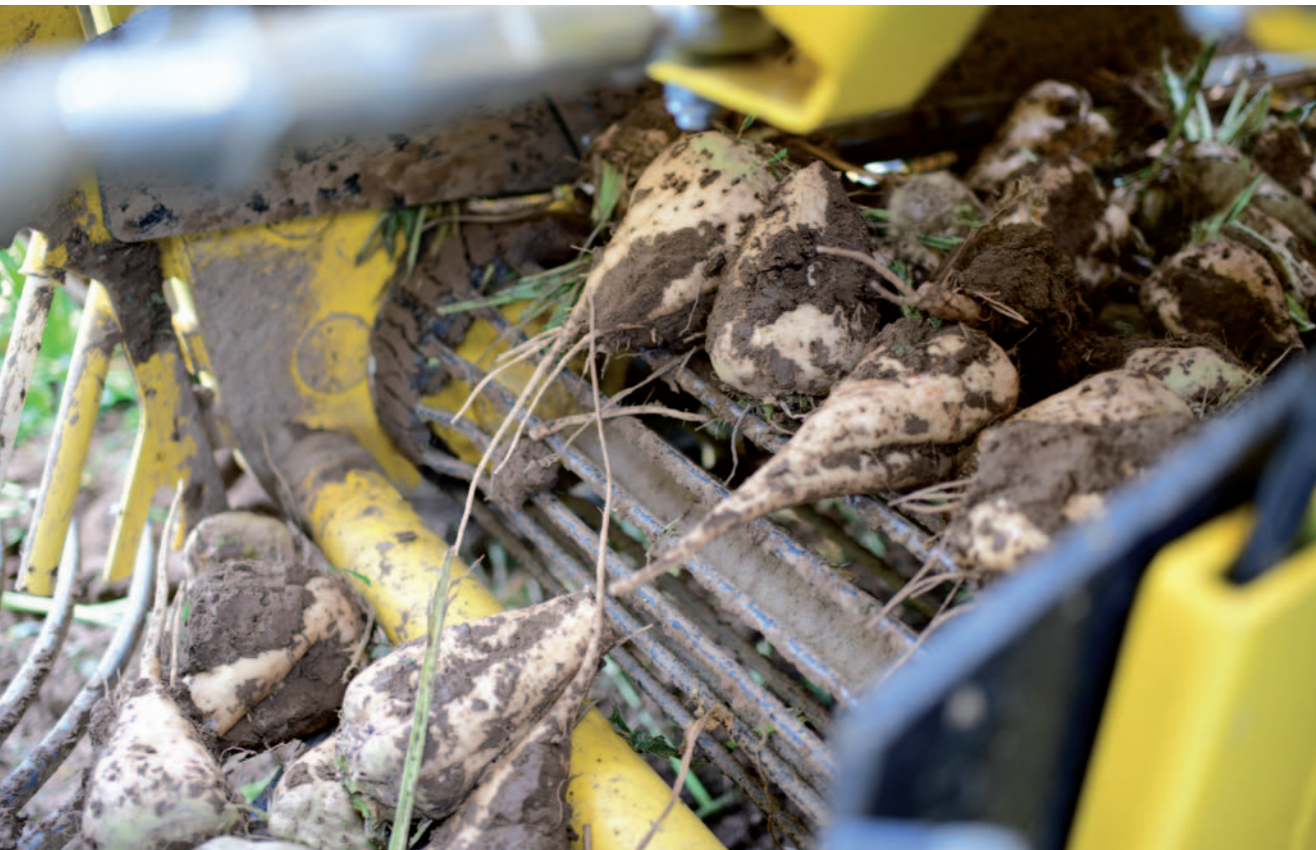
Rotating transition tubes at the elevator infeed prevent accumulation of soil
