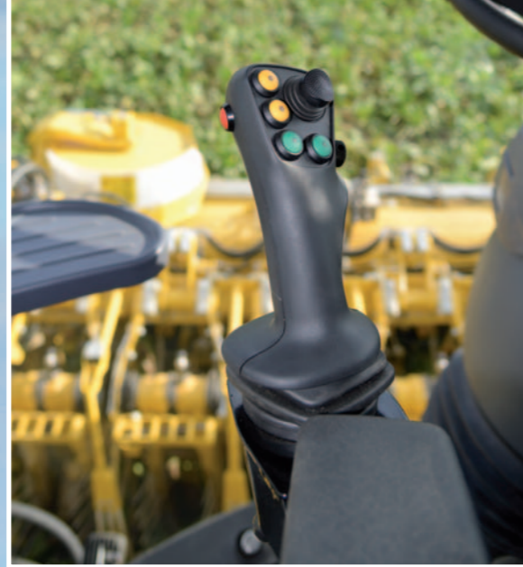
Control element on the left armrest for fine control of bunker unloading
